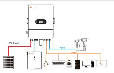
Figure 2.1-1 Block diagram of hybrid solar inverter system
