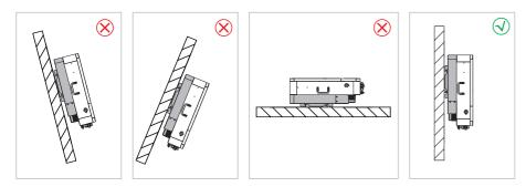
Figure 3.3-2 Installation position
