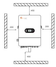
Figure 3.3-1 Installation space of one inverter
