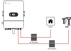
Figure 4.3-2 Ac breaker connection
