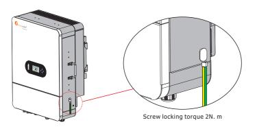
Figure 3.4-3 Rack earth(Ground wire locked by M5)
