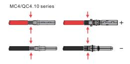
Figure 4.1-2 PV cables to PV connectors
