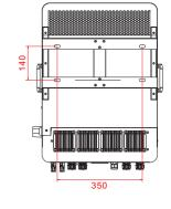
Figure 2.2-2 Inverter dimensions
